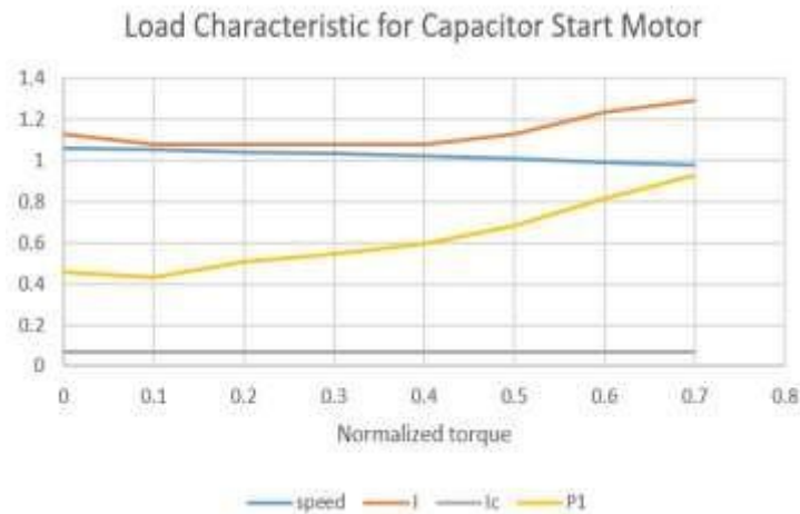
Figure 4:load characteristic for start motor
