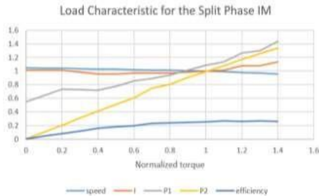
Figure 8:load characteristic for split phase IM
